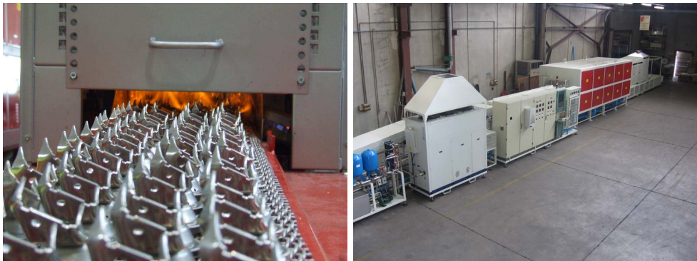
Figure 3: Example of arrangement of the pieces on the conveyor at the furnace inlet (left) and picture of a complete furnace line (right) installed at Borgwarner Emissions Systems Spain S.L. Company.
